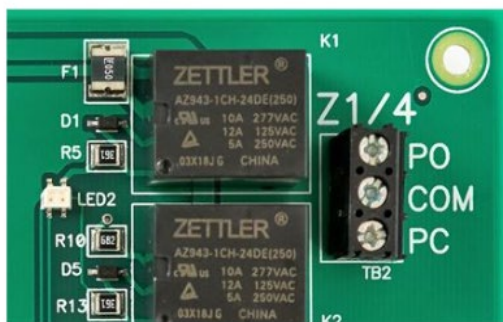
Zone panel damper connection terminals
